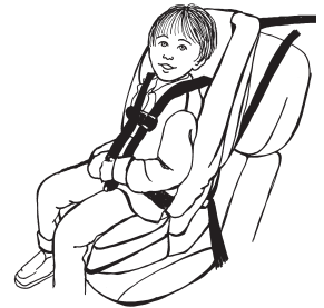
Car seat for child over 40 pounds, used with seat belt and tether
