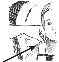
D. Check harness tightness. If you can pinch any slack, it is too loose.
